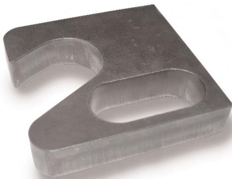
3/4" (20 mm) Mild Steel Cut Sample
