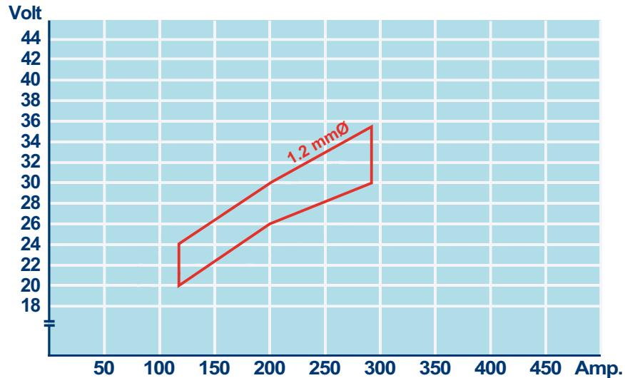
Note: The above parameters are typical range for DW-310 with mixed gas. Adjust voltage for 100% CO<sub>2</sub>.
