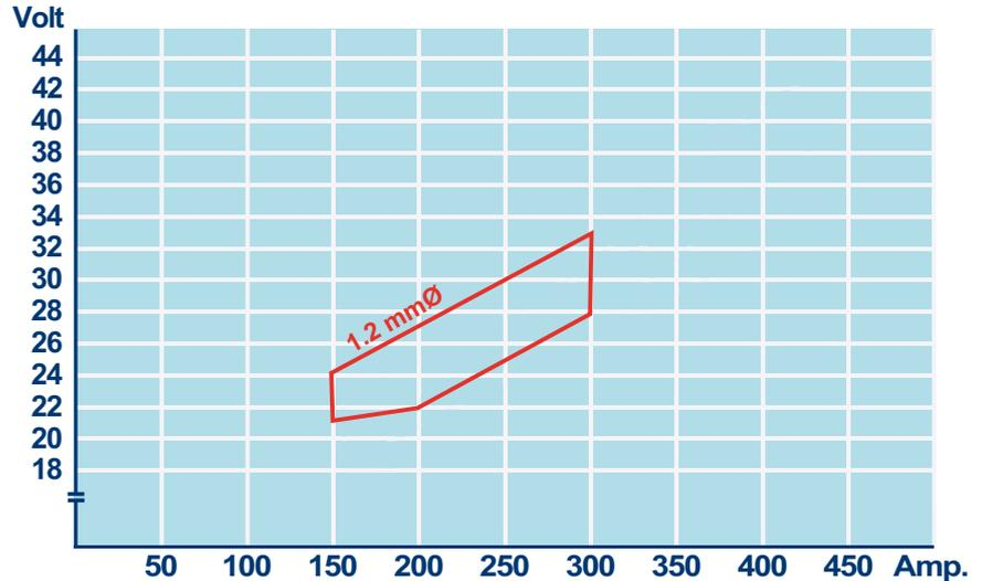
Note: The above parameter ranges are intended for Ar+CO<sub>2</sub>. More voltage is necessary for 100% CO<sub>2</sub>.
